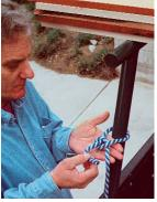
**1**. Start with a bowline, tied to the rack. Then lead the line over the load and back.
