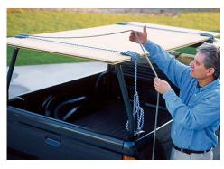
When carrying a mixed load, it's safest to tie down the plywood first. Pad the edges with carpet scraps or cardboard to avoid damage.
