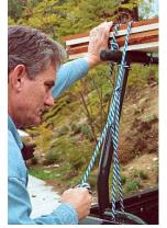
4. Then pull down hard. Try to move the lumber sideways; if it moves, pull harder on the rope.
