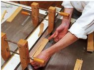
Using stop blocks, make a rip cut along the rabbet to remove the center portion. Be sure to stop short of the notches. Finish the rip using a handsaw.
