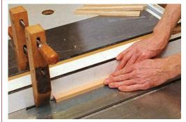
Stopped rabbet engages locking tab of lower slide. The rabbet, <sup>1</sup>4 in. wide by <sup>5</sup>/<sub>16</sub> in. deep, runs two-thirds the length of each upper slide.
