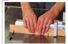
Set the tablesaw blade for a  $rak{1}{2}$ 6-in.deep cut. Make crosscuts 15/16 in. from the front and 11/4 in. from the rear of the lower slides. Left and right slides are mirror images of one another.
