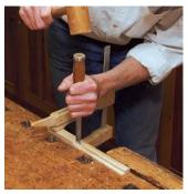
**Square the corners of the stopped rabbet.** Remove the waste using a chisel.
