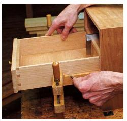
After installing the slides in the case, mark the cleat locations on the drawer. Clamp the drawer at full extension and trace along the step and lower slide.
