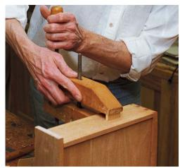
**Cut mortises into the drawer sides.** Once the cleats have been glued in place, the drawer is ready to be used.
