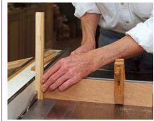
**Cut a notch at the rear of the upper slide.** The notch is 1 in. from the back and as deep as the rabbet.
