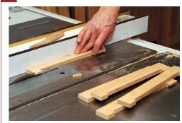
Remove the upper step at the front of the slide. The step is removed right down to the base of the rabbet.
