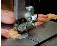
Remove the waste behind the notch. The locking tab engages with the upper slide and keeps the drawer from tipping.
