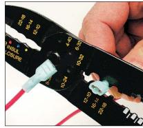
Sensor and relay have ½-in. spade lugs. Female connectors are attached to the wire with a crimping tool.
