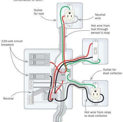
fuse. Normally, the up position means "on." The wires used to connect all of the parts have to be large enough for the circuit breaker that powers everything. Twelvegauge wire is the minimum size required for a 20-amp circuit.
