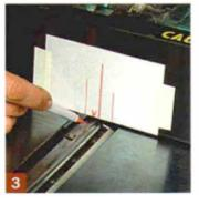
Using a ruler, split the distance between the marks to locate top dead center. Place another mark to indicate where the cutterhead slot lines up.
