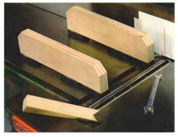
Bar magnets (available from hardware or electronics stores) glued to a block of wood (do this on a level surface) with silicone adhesive make a decent knife holder/straightedge. Tighten the bolts on the locking bar so that each knife (at top dead center) is level with the outfeed table.
