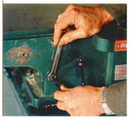
infeed tables have one gib each with two or three adjusting screws. Loosen the locknut and snug up the Allen-head screw to take up any slop. Tighten the screw nearest the cutterhead a tad more than the bottom one.
