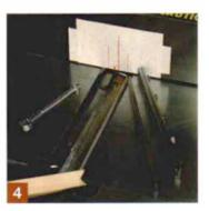
Align a knife to top dead center and wedge the cutterhead in place. Loosen the locking bar bolts and replace one knife at a time.
