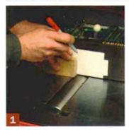
First find top dead center of the cutterhead: Slide a flat block of wood with a projecting screw head until the screw butts up against the cutterhead.
