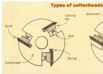
Some cutterheads use springs to adjust knives up or down. A clean shop floor will help ensure that you can track down an AWOL spring that will inevitably roll off the table.
