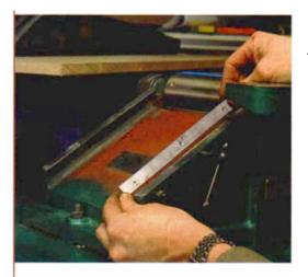
You need not disassemble a jointer to do a tune-up. The narrow. flat bar is a gib, which takes up wear in the dovetailed ways of the infeed and outfeed tables.
