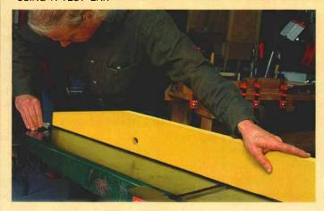
Use the test bar and feeler gauges to check the tables for flatness. Tables may sag over time. New machines, however, may be out of adjustment, too.
