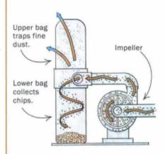
BARREL-STYLE TWO STAGE The larger chips entering a two-stage collector tend to drop out before they have a chance to strike the impeller.
