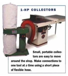
same machine, rated at 650 cu. ft. per minute (cfm) by the manufacturer, but when hooked up to 6 ft. of flexible hose, it moves about 420 cfm. That's slightly less than the 500 cfm recommended for a 15-in. planer, but 90% of the time the 1-hp collector can handle it because I rarely plane 15-in.-wide stock.
