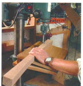
Connect two pieces of plywood with a piano hinge. Fit a wood wedge between the leaves to create the angle needed.
