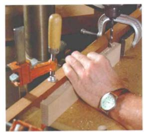
By trapping stock between two stop blocks, a mortise can be roughed out using a brad-point bit.
