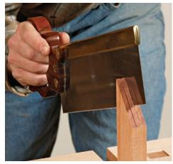
**Cut the cheeks with a backsaw.** Then remove the waste with a coping saw.
