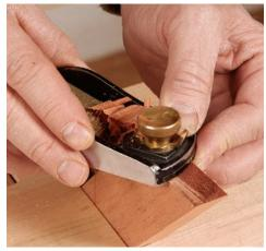
**True the miter.** The low-angle, bevel-up blade of a block plane severs the end-grain fibers cleanly. Keep an eye on the layout lines on both faces.
