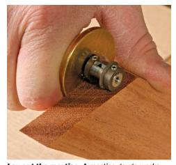
Lay out the mortise. A mortise gauge works best for this, because it marks both sides at once. Cut along the end grain, then down the outside edge. Do not change the gauge's setup.
