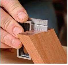
**Check for square.** Use a small square to check across the miter, then pull out a combination square and check the miter's angle. Refine as needed.
