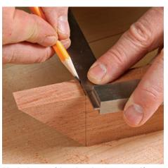
**Mark the outside edge.** Don't use a knife here, because the severed fibers would be visible.
