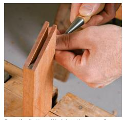
**Pare the bottom.** Work into the center from both edges. The knife line cut earlier on the inside edge allows the fibers to break off cleanly rather than tear out.
