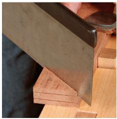
**Then cut the shoulders.** Don't rely on the saw for accuracy. Cut rough and then pare to perfection.
