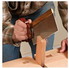
**Cut the cheeks first.** Start at the top corner of the inside edge and hold the saw at a roughly 45° angle.
