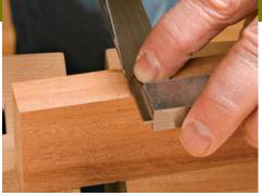
**Knife across the inside edge.** To align the square, place the knife in the line cut into the face and slide the square up to it. Mark the edge, then mark the second face.
