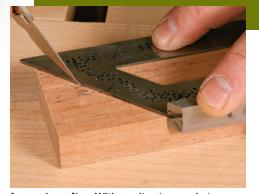
**Lay out a miter.** With a miter (or combo) square aligned with one corner, strike a knife line across the face of the stile.
