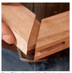
**Beautiful and strong.** After fitting the cheeks, the joint should come together snugly, with a tight miter where the parts meet.
