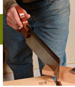
**Remove waste with a backsaw.** This cut is for roughing out the angle, so be close to the line, but not on it.
