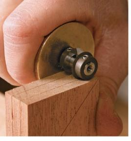
Use the mortise gauge again for the cheeks. To ensure that the tenon aligns with the mortise, register the fence against the same face on the rail as you did on the stile.
