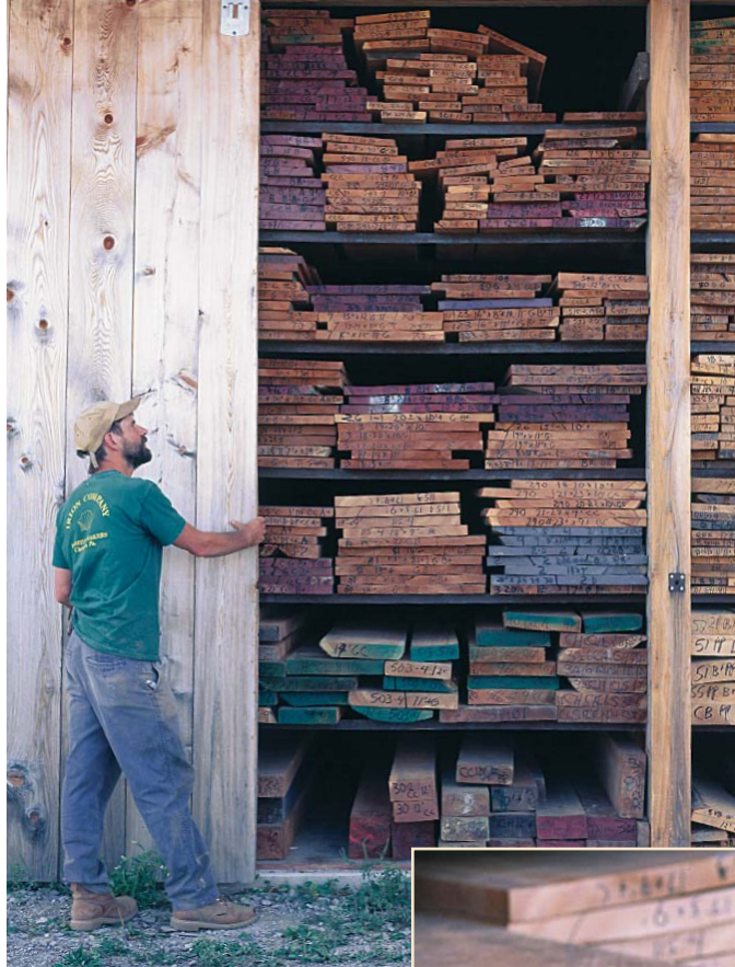
The Louie decimal system. The author's code tells him this board is one of a set of five cut from log No. 2; it is 19 in. wide; it has two clear 5-ft. cuttings and a 3-ft.-long section that will yield excellent drawer fronts; it is curly cherry; and it rates an A-minus for figure.
