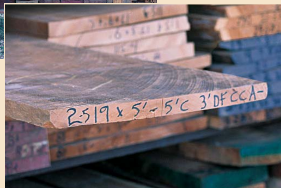
The Louie decimal system. The author's code tells him this board is one of a set of five cut from log No. 2; it is 19 in. wide; it has two clear 5-ft. cuttings and a 3-ft.-long section that will yield excellent drawer fronts; it is curly cherry; and it rates an A-minus for figure.
