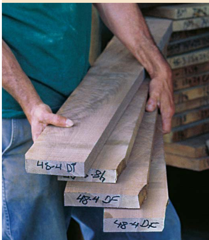
The Louie decimal system. The author's code tells him this board is one of a set of five cut from log No. 2; it is 19 in. wide; it has two clear 5-ft. cuttings and a 3-ft.-long section that will yield excellent drawer fronts; it is curly cherry; and it rates an A-minus for figure.
