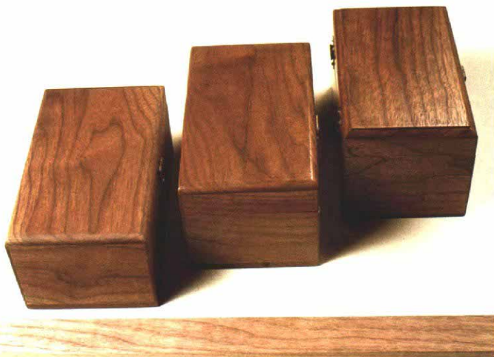
Same wood, different lusters —These three boxes were made from a single piece of walnut (a strip is shown at bottom), but finished differently: The left box was coated with linseed oil to give a dull look; the center box was wiped with shellac and waxed to a satin sheen; the right box (with the reveal on the lid) was brushed with polyurethane varnish and burnished to a low gloss. The finishes also bring out variations in color and grain contrast.
