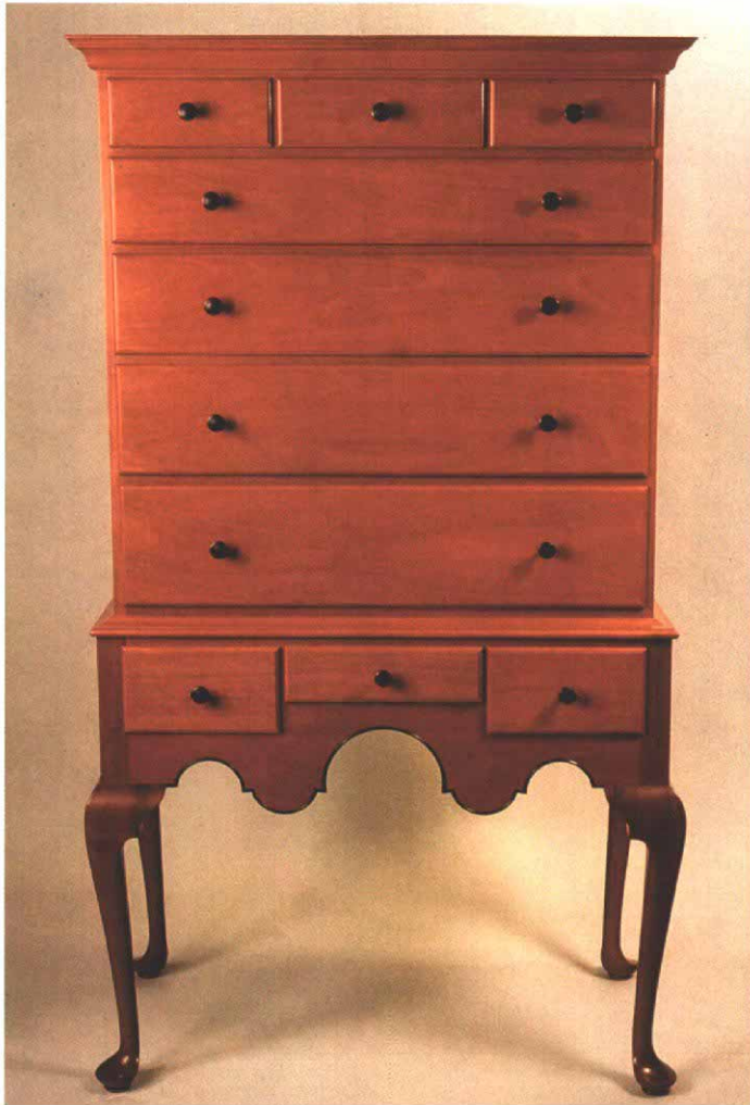
Highboy gets a high-end finish. Andrew Davis of Santa Fe, N.M., hand-rubbed layers of lacquer to finish this mahogany Queen Anne highboy. Aniline dye and japan colors were used to add tint.
