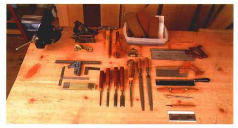
A basic kit of hand tools doesn't have to cost a fortune or take up a lot of space. Here, with some changes and additions, is Mario Rodriguez's basic kit. The chisel handles (and the brass-backed dovetail saw's handle) are all replacements made by Rodriguez.
