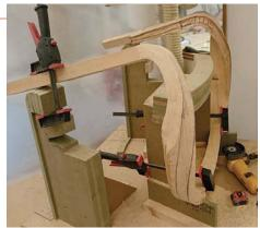
**Freehand shaping.** Smith used an angle grinder for some of the shaping and rasps, files, and spokeshaves for the rest. A tent of plastic sheeting contained the dust.
