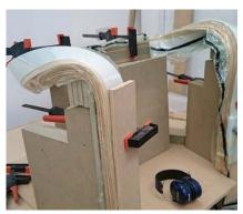
**Major bending.** Smith built MDF forms to bend the chair parts. Applying epoxy to all 80 strips in the front leg-and-arms component and clamping it up took three hours.
