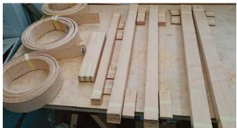
A chair frame in the raw. Straight-grained, flitch-cut European ash veneer, 0.6 mm thick, was used for the frame (left). After ripping the sheets into strips and cutting them to length, Smith sorted and numbered them to keep them in the order they came from the tree (above).
