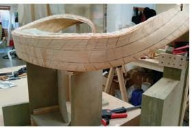
**Out of the bag.** Once the epoxy cured, Smith used hash lines to indicate where wood should be removed during the initial shaping.
