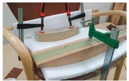
Final fitting. Using the threaded studs, Smith epoxied the seat and back to the chair frame.
