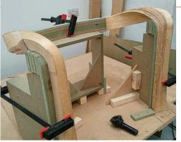
**Square before circle.** Smith cut the components to a square section before shaping them round. He made some cuts with a saber saw, others with an Arbortek angle grinder with a planer head.
