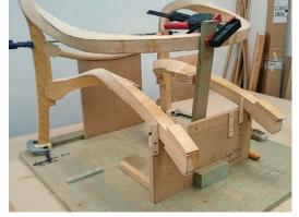
Ready for the router. A curved template guides the router in cutting the male half of the back leg joint.
