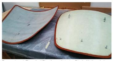
**Two-part seat.** The paired fiberglass substrates, fitted with threaded steel studs for attachment to the frame, were trimmed to size and then upholstered with leather.
