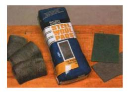
The next step depends on the finish I'm using. I put oil on most of my work (except tabletops.) because I like the way it allows the texture of the wood to be seen and felt. When finishing with oil, I stop at 150-grit. Oil is a penetrating finish, and the finer you sand, the less penetration you obtain. I apply the first coat (which does the most penetrating) before I go to finer abrasives.
