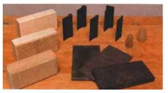
Always sand with a cushion to keep your surface flat. Cork blocks, cork-faced blocks and rubber sanding pads all will work. The rubber Tadpoles (right, background) allow sanding of concave and convex moldings, and the finger rubbers protect the fingers while providing a good grip on the sandpaper. The solid wood block is useful as a backing for the nylon abrasive pads.
