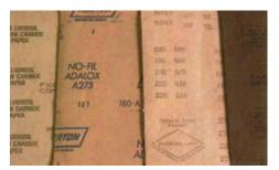
Allyou need to know about a sandpaper is printed on its back. Manufacturers usually indicate grit, coating density (open or closed coat), backing weight and sometimes other information, such as whether a no-clog coating has been used, as is the case with the first (Lubrisil) and second (No-Fil) sheets above.
