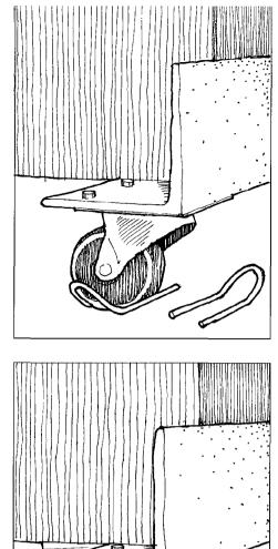
**Hinged dollies** are what stagehands use to move props and scenery. The basic method is to attach the wheels to a plywood plate and then to hinge the plywood to the base or legs of the machine. Two versions are shown below.
