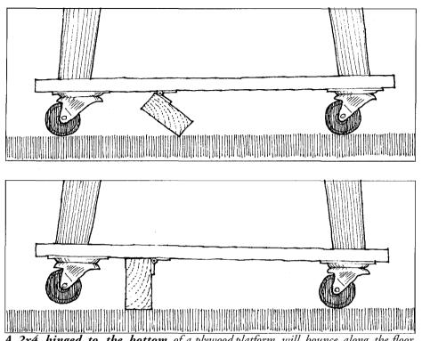
A 2x4 hinged to the bottom of a plywood platform will bounce along the floor when the tool is rolled in one direction. When you want to park the tool, just lift it slightly, and then rock it up onto the 2x4. Hinge the 2x4 so that the hinged joint resists the thrust of feeding material.
