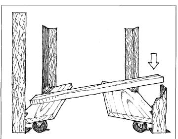
In this arrangement, a single lever can activate two sets of hinged casters.
