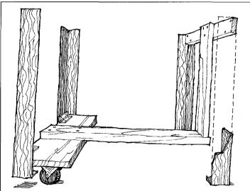
Pressing down on the lever deflects the latch. When the lever clears the latch, the latch springs back and locks the wheels in the down position.
