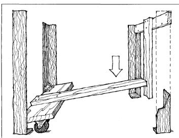
A simple latch activates this two-wheel dolly. The horizontal lever is screwed to the hinge plate. The vertical latch is screwed to a crosspiece or to the machine itself.
