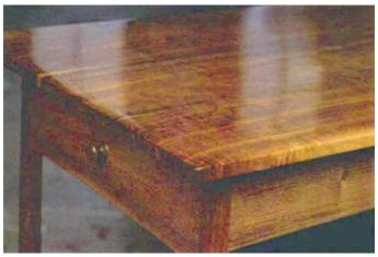
The hue of sun-bleached walnut suited the author, but the tabletop needed work. Using mineral oil and rottenstone, he rubbed out numerous minor scratches and scuffs, as well as gave the surface a new shimmer, without changing the color of the wood.
