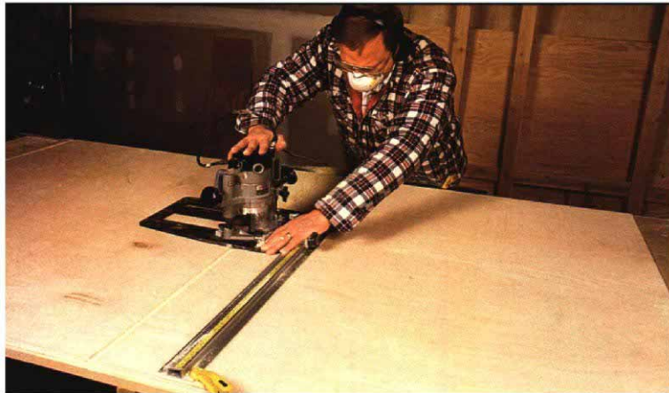
To rout dadoes across panels with Exac-T-Guide, clamp the T-square in place at both ends, and slide the router on the mounting plate along its long arm, as shown. Exac-T-Guide is the only unit that has a stock mounting plate that accepts a wide variety of tools.
