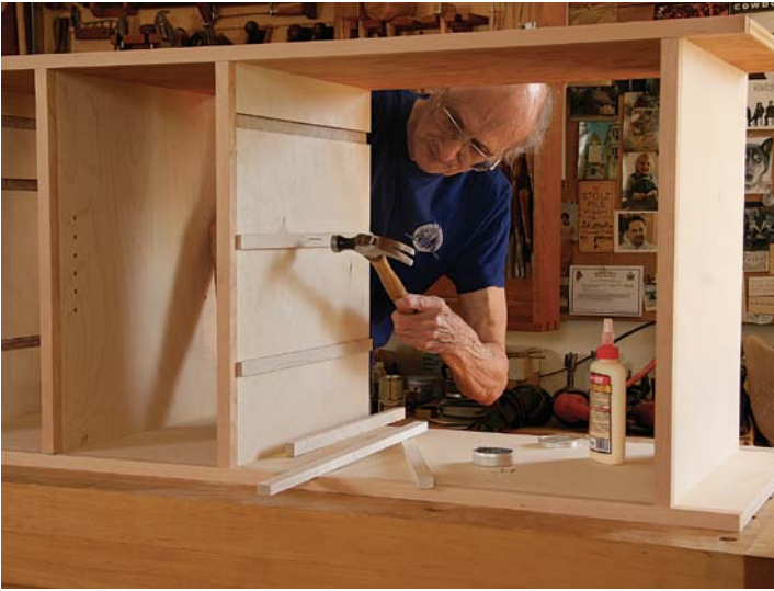
Fix the runners. Becksvoort glues in the maple runners, using brads instead of clamps to hold them in place.
