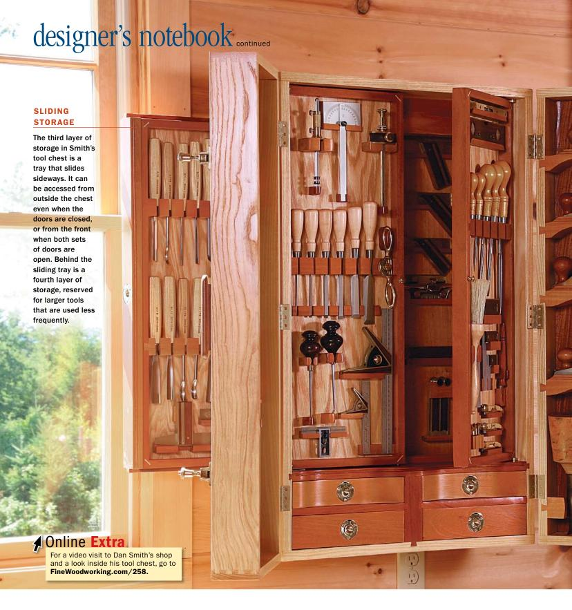
When you do slide the tray aside, it travels right out the side of the chest. This means you can also access the tools in the tray without ever opening the doors: Just pull the brass ring on either side of the chest, and the tray slides out. The wooden handle on the front of the tray acts as a stop, so the tray slides just halfway out either side of the chest.
