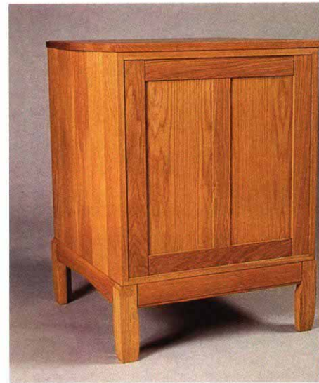
Above: This white-oak file cabinet was made with a variety of router shaping and joinery. Its boxy appearance is softened by recurring triangular designs that appear in the inlaid drawer fronts and the top, in the shape of the aprons and overhanging top edges, and in the routed detail on the side panels.
