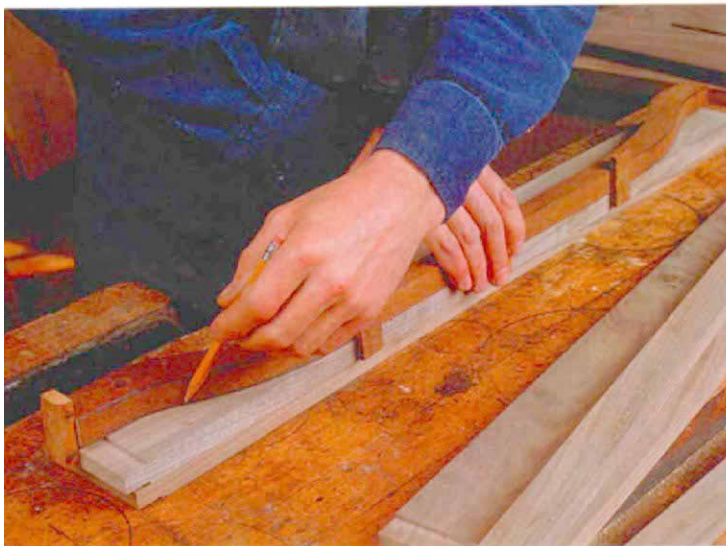
Below: Mehler traces a side rail from a pattern that has stops on its side and end. This way he can locate the rail on the workpiece.
