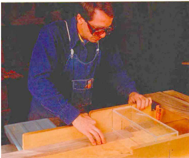
Above: The author crosscuts shoulders on the stretcher and rails by using a sliding table with a stop set for the tenon length.
