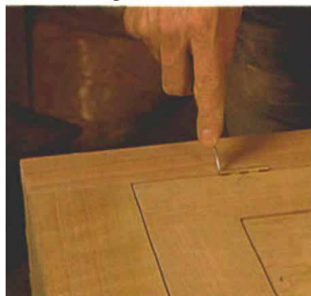
With the door positioned, Becksvoort uses a knife to transfer the hinge location to the face frame. For accuracy, you must not move the door when making these marks.
