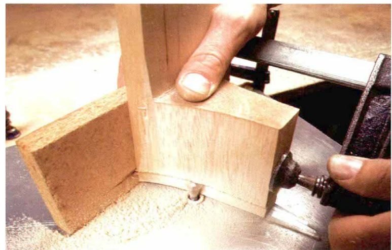
The dovetail that joins the guitar's neck to the body is shaped on the router table. A standard dovetail bit cuts the male dovetail as the neck, screwed to a Plexiglas template that rides against a stationary guide bushing, is moved over the table.
