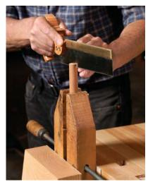
Perfect for small or odd-shaped parts. Getting a steady hold on turned or round work can be tricky. Adding notches to hand screws is an easy and secure way to hold round stock at the bandsaw (above) or upright in a bench vise (left).
