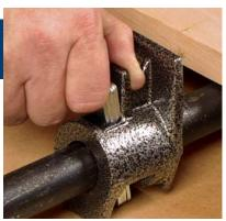
Cheap and versatile. The head of the pipe clamp threads onto the end of the pipe, while the tail (above) slides on and retains its position with a plate clutch. The pipe comes threaded at both ends, so all you need to create a longer clamp is an inexpensive coupler and another length of pipe (right).
