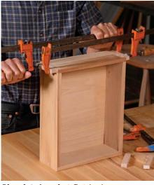
Pinpoint clamping. F-style clamps are great for smaller jobs that don't need high pressure or large clamps, such as gluing up a drawer (above). Versions with an extradeep throat make it easy to clamp jigs to benchtops and work surfaces (left).
