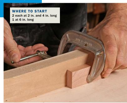
C-clamps are always useful to have around, mostly because of their good functionality and low level of fussiness. They're small but strong and are unlikely to distort under pressure. They are used for a variety of tasks, but are especially useful for clamping down stops on tablesaw sleds and other jigs with a fence, or any small jobs where an F-style clamp would be unwieldy.
