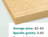
Percent shrinkage: Tangential 7.8, Radial 4.9 T/R ratio 1.6
