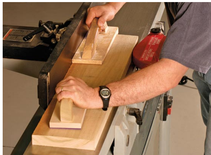
Use a pair of push blocks for face-jointing. It's best to have a nonskid block at the board's leading edge and a cleated block at the rear.
