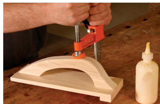
Easy to assemble. A cleated push block can be made in less than 15 minutes. Because the glue joint is long grain to long grain, screws are not needed.
