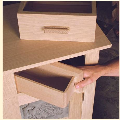
**Nothing complicated here.** After one drawer is removed, the hidden compartment, which rests in a dead space between two drawers, may be pulled out.
