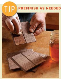
Shellac dries fast, so you can finish parts without slowing down assembly. This means you can prefinish components like these dividers that would be hard to reach after glue-up.
