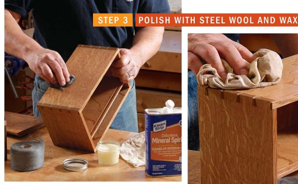
**Smooth and wax in one step.** The steel wool and wax combination levels any dust particles and produces a satin finish that's friendly to the touch. Wet the steel wool with some mineral spirits and then dip it into the wax. This will make it easier to apply a thin, even coat. Once the wax has dried, buff out the piece with a clean cotton rag (right).
