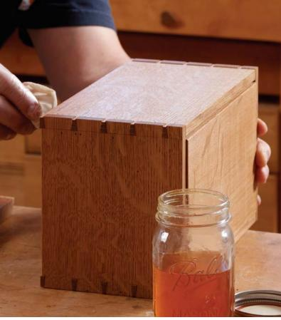
**Stop before the finish gets too thick.** Pekovich applies coats until the surface is just a bit glossier than he wants in the finished product. This will ensure adequate protection without building too thick of a film finish.
