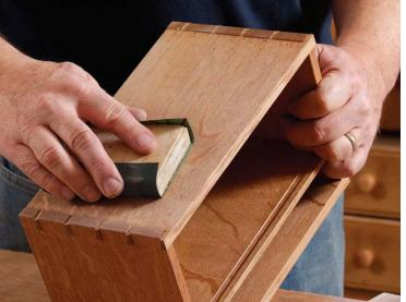
Start with a good base. The first coat, called the washcoat, seals the fibers and raises the grain. This coat will get sucked into the wood and dry quickly. After the washcoat is dry, use the highest-grit paper that you used for prep to knock down the raised grain.
