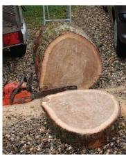
From log to lathe. After chainsawing a thick disk from the log, Oudet turns a tenon to fit his chuck, then turns the outside face flat.
