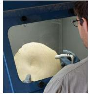
It's a blast. After air-drying for several days, the disk goes into the sandblaster. It can take three days or more of sandblasting to achieve the transparency Oudet is after.
