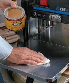
Make surfaces slick. Wood passing under the rollers applies a considerable amount of friction and pressure to the bed and tables. Applying wax to those surfaces will prevent things from bogging down.
