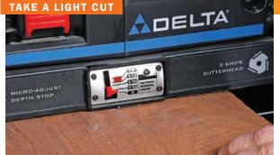
Lighter is better. Set the depth of cut for less than 1/16 in. to reduce the likelihood of tearout. This is especially important on wide stock, which can bog down the smaller motors on benchtop planers.
