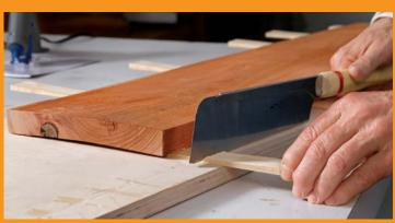
**Trim the shim.** Cut the shims with a handsaw, making sure they're well inside the edge of the sled to avoid any hangups as the sled passes through the planer.
