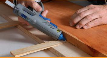
**Keep the shims in place.** To keep the shims from shifting while the sled is inside the planer, use hot glue. A single, thick bead where the shim and board meet is usually enough to hold it down.
