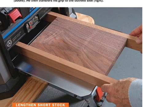
**Add some runners.** For stock that's too short to plane, glue hardwood runners to the edges. This effectively increases the length of the board so that it can be grabbed by both feed rollers, as well as keeping snipe from the short length of material.
