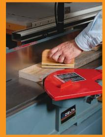
The planer doesn't flatten a board; it creates a surface that's parallel to the surface riding against the bed. One side of the board must be flattened at the jointer first. That flat face is the surface that rides against the bed.
