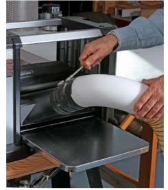
**Use dust collection.** The chips created by the planer are not only hazardous to your health, but they also can get trapped under incoming stock and cause an irregular cut with poor results.
