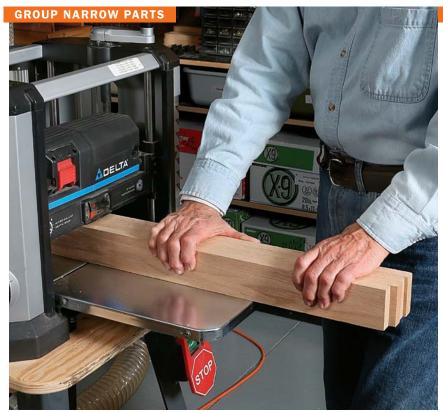
**Planing on edge.** When you need consistent and dead-accurate widths for multiple components, edge-planing gives great results. As he feeds the parts into the planer, Forshee holds them firmly to keep them upright and together in the center of the bed (above). He then transfers his grip to the outfeed side (right).
