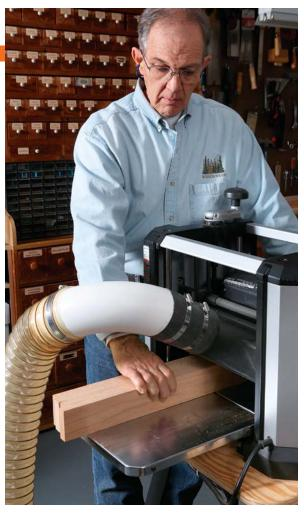
can be reduced by feeding boards through the planer butted end to end. This keeps the feed roller tension equalized. This "planer train" technique can also be used to control shorter stock.
