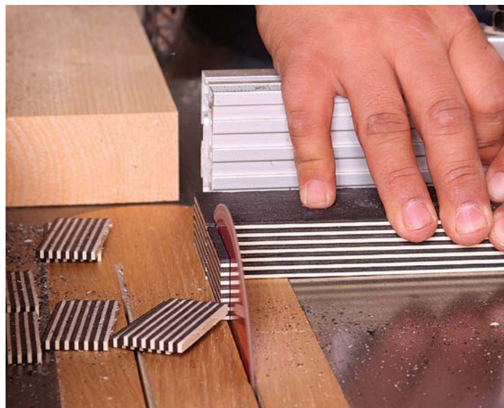
Chips from a brick. After ripping the brick to width, crosscut 1/8-in.-thick chips from it. Use a zero-clearance insert, a stop block, and the miter gauge.
