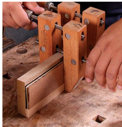
Simple jig for glue-ups. Roman coats the outer layers of veneer with liquid hide glue, then uses an L-shaped MDF jig to keep the parts aligned when clamping.
