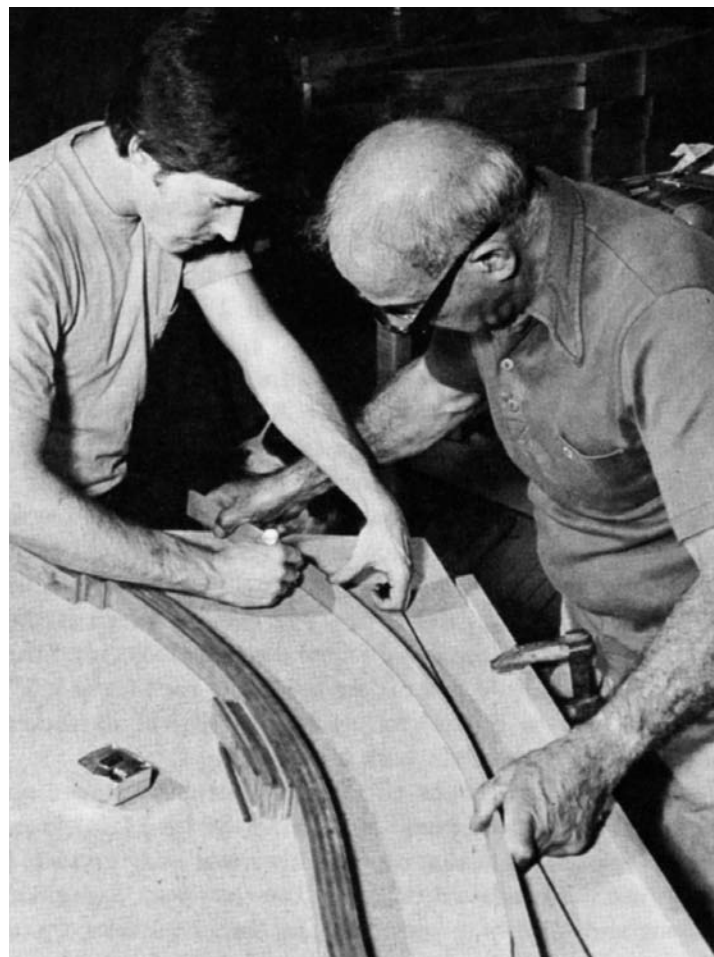
With assistant Mike Johnson tracing the curve, Maloof demonstrates how he casts the shape of a rocker on the piece of particleboard that will be its gluing form. Also shown is the glued-up blank, with platforms for smoothing the transitions between legs and rocker, ready for shaping.
