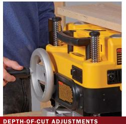
Convenience is king. A depth-of-cut adjustment wheel on the side is easy to reach. Three of the machines have side-mounted wheels, but this convenience doesn't trump surface quality.
