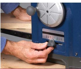
**Depth stops simplify repeat milling.** Stops for common thicknesses make it a snap to mill parts to the same thickness, a handy feature when you need to remake a part. All the stops tested were accurate.
