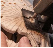
**Leave the lines.** Depending on the size and design of the carving, Layport uses either a standard jigsaw or this lightweight gourd saw to cut out the waste.
