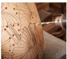
**Drill holes for access.** To prepare for sawing out the shapes, Layport drills access holes big enough to fit his jigsaw blade.
