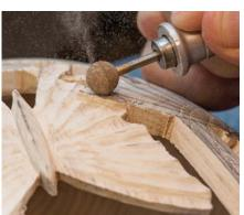
The rotary arrives. After sawing, Layport shapes the piece using rotary-tool cutters, burrs, and sanding attachments. He also uses files and rifflers.
