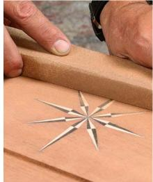
The pointers usually don't need much fitting. Slide the point end into the recess and see how far it will go, checking the fit along the sides. As you fine-tune the sides, try not to change the width at the fat end, where the two triangles will meet. If you have to trim the fat end, make sure you take the same amount off both sides, and do the same to the inner triangle piece afterward. When planing the tip, take the same amount off both sides so the ebony/ holly joint stays centered.
