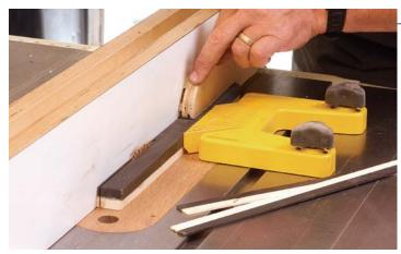
**Slice up a two-color blank.** Start by gluing up an ebony and holly sandwich using epoxy. After squaring two faces on the jointer, Fitzpatrick saws off <sup>1</sup>/<sub>8</sub>-in.-thick slices, using a thin-kerf blade to minimize waste.
