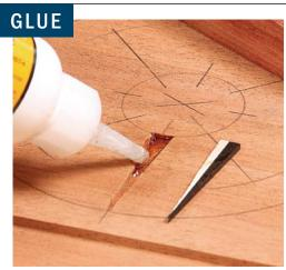
**Cyanoacrylate works best.** Use mediumviscosity glue, and spread it in the entire recess.
