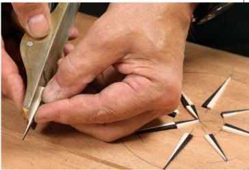
**Shave to the line.** Rub the parts on a block plane or sanding block to trim them to the layout marks and a sharp point. Place them on the workpiece to be sure all of the fat ends match.
