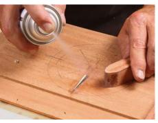
**Press it down and zap it with activator.** Fitzpatrick uses the flat side of a stick to press the inlay down, and then the rounded end to be sure it is fully seated. The activator spray cures the CA glue instantly, letting you move on just as fast.
