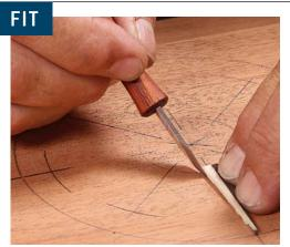
**Align and scribe.** Use the centerline of the triangle to align it. Then hold it in place and knife gently around it.
