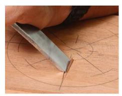
**Cut the recess.** For small pieces like these, it is all chisel work (plus an X-Acto knife). For larger pieces, start with a trim router and a small bit. The goal is to leave the inlay a little proud, so it can be leveled later.
