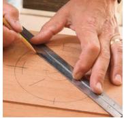
Divide a circle and connect the dots. Draw the largest diameter and mark the east/west layout lines. Then use dividers to mark out eight equal divisions. After drawing the small circle, connect the dots to indicate each pointer.
