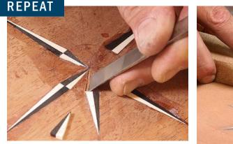
**Now do it 15 more times.** The reason for doing each pointer one at a time is so the fragile grain at the center of the panel is always supported on all sides. A long sanding block, used in the direction of the panel's grain, levels the inlay and preps the panel.
