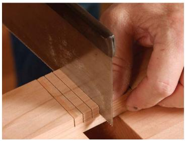
**Kerf the waste.** The more kerfs you make the easier it is to remove the waste afterward. A kerf every  $\frac{3}{6}$  in. to  $\frac{1}{2}$  in. works well.
