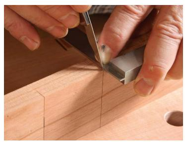
**Come down the edge.** Transfer both shoulders halfway down on both edges. Make sure to cut a clean, deep line.
