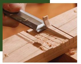
**Be aggressive.** Using a wide chisel, whack away the waste as quickly as you can, but always work in toward the center and cut gently upward.
