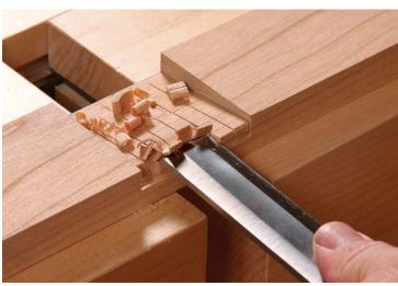
**Work from the opposite edge, too.** Again, take out chunks of waste, but also angle the chisel gently upward, leaving a short peak of waste in the middle.
