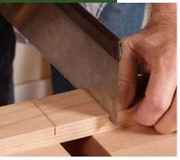
**Cut both shoulders with a backsaw.** Start just like you did with the half-lap, by paring a groove along the shoulder lines that can be used to guide the saw.
