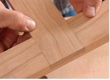
**Strong and gap-free.** Accurate layout and smart paring pay off again. There are no gaps at the shoulders and the depth is spot-on.
