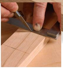
**Back to the square.** After putting the knife back in the tick mark, slide the square against the blade and cut the second shoulder.
