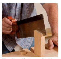
Flip and repeat for the opposite edge. After you've cut down to the shoulder, bring the saw horizontal and cut away the remaining triangle of waste.
