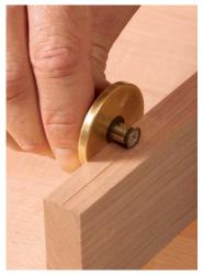
Use a marking gauge for the cheek. Scribe a line in the exact center of the part's thickness. Mark the end grain as well.
