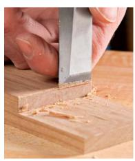
Work down on the shoulder. Place the chisel into the scribed shoulder line and push down. Use one hand to keep the cutting edge in the scribe line.
