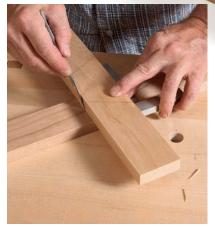
Mating piece determines width. Place it against the blade of the square and then use the knife to make a small tick to mark its width.
