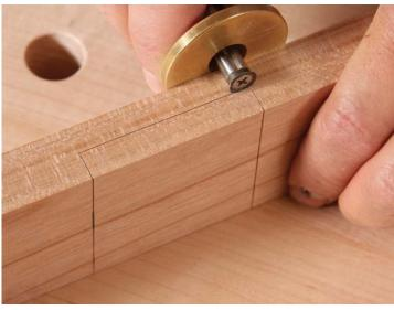
**Scribe the depth.** The marking gauge should be set for half the thickness.
