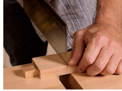
**Cut the shoulder to depth.** The saw's teeth should just kiss the vertical wall cut by the marking knife. Keep an eye on both edges of the part so that you don't cut below the cheek line.
