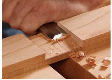
**Remove the peak.** Work in from both edges until the bottom is flat. For the final passes, put the chisel into the scribe lines before pushing inward.
