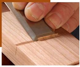
**Cut a groove at the shoulder.** With a wide chisel ½s in. from the shoulder line, cut down to the scribed shoulder, creating an angled notch.
