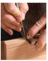
Wrap it around the edge. To locate the cut, put the point of the knife in the kerf and bring the square up to it. Scribe halfway down the edge.
