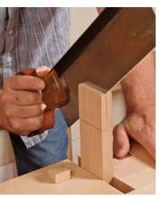
Make a diagonal cut down one edge. At first, follow only the vertical line on the part's edge. Then come in across the board's width until you reach the halfway point.
