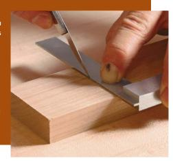
**Mark the shoulder.** Use a square and knife to get a clean, deep (1/2s in.) cut across the grain. The width of the mating part determines the shoulder's location.
