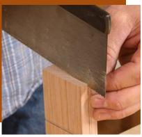
**Create a shallow kerf on the end grain.** Start at the far corner using the scribed line as a guide. Cut just a bit deeper than the teeth.
