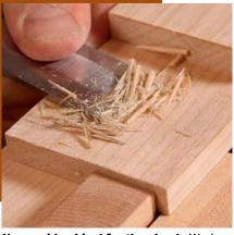
**Use a wide chisel for the cheek.** Work from the edge toward the middle, then turn the part around and come in from the other edge. Pare down to the scribe line.
