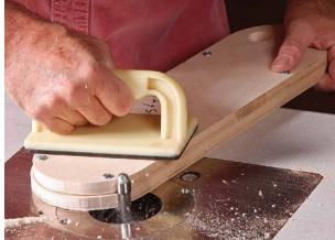
**Use the original as a routing template.** After roughing out the master blank, screw the original insert to the blank. Then use a flush-trimming bit at the router table to get a perfect replica (left). A wood filler strip in the open end of the insert prevents the bit from catching. Once the master is done, screw it onto another blank to make more insert blanks (right).
