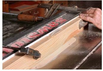
½-in. plywood will be just below the top, and will need to be raised flush. For that job, I use ¼-20 Allen leveling screws. I drill and tap through-holes for those screws so that I can adjust the height quickly while the insert is in place.
