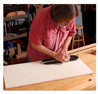
A simple tracing. Use the plate that came with the saw to transfer the outline to the plywood.
