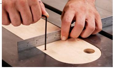
Get the inserts flush with the table. Using a straight rule and Allen key, bring the plate up until it's flush against the ruler and doesn't rock on the adjusters.
