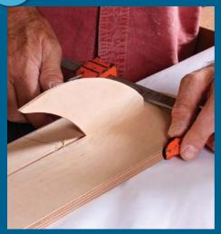
If your saw doesn't have a splitter or riving knife, you can add a shopmade splitter by routing out behind the blade and gluing in a piece of ½-in. plywood. Van Dyke installs an oversize splitter so that when the blade is raised, it will cut the splitter to perfectly match the blade.
