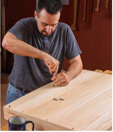
The rest of the backboards. Note the screwing pattern, designed to hold down the backboards while letting them shrink and expand. The bottom board is fully screwed and glued, like the top one.
