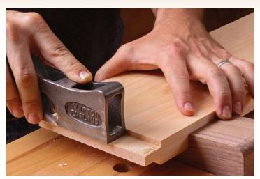
**Use a shoulder plane to fit the cheeks.** Do most of the planing on the front cheek, so you don't change the distance at the back. Then notch the ends to cut the tenon to width.
