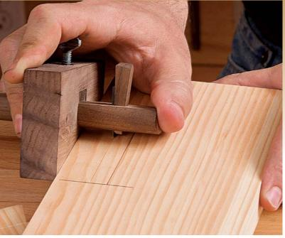
**Scribed layout makes for cleaner cuts.** Use a marking gauge to scribe the sides of the mortise. Scribe the corresponding line on each case side before changing the setting on the gauge.
