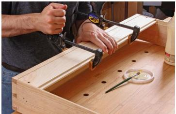
Glue in the top backboard and the shelf. Screw it into place at the ends, but also clamp across it to strengthen the glueline at the top edge (above). Now glue and clamp on the screw-strip doubler while it is easy to access, and then rip the shelf to width and glue it in (right).
