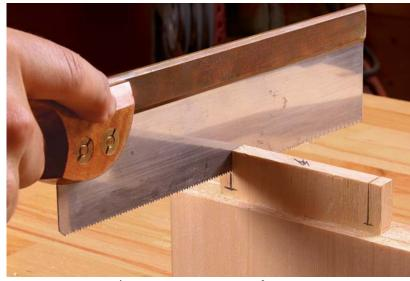
**Kerf the tenons.** Saw  $\frac{1}{4}$  in. from the ends and stop  $\frac{3}{46}$  in. short of the shoulder.
