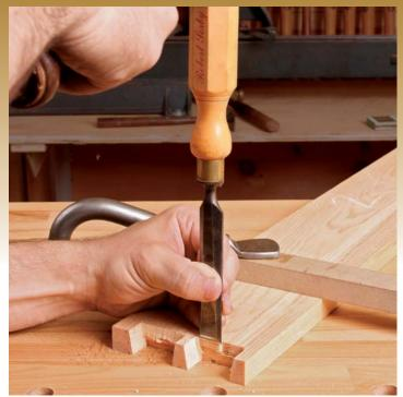
Pins first. Faia cuts his dovetails pins first, sawing right to his pencil lines. He uses a coping saw to remove most of the waste, and pares to the baseline with a wide chisel as shown, working in from both sides.
