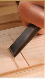
Ramp the scribe lines. Take an angled chip along the inside edge of each line. Do the same at the stopped end.
