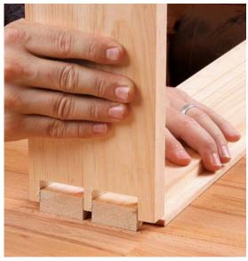
Pine is forgiving. After sawing the tails right to the lavout lines, vou shouldn't have to pare them. But if you do, pare sparingly with a wide chisel.
