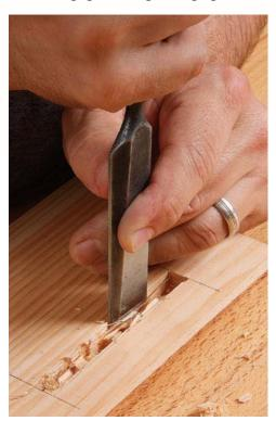
**Drill and chop.** After drilling out the waste, do most of the chisel work from the outside face, which is the most important. Work slowly back to your scribe lines.
