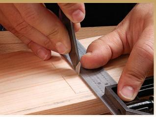
**Scribe the edges.** Dry-fit the case and measure from the top to mark the first edge. Use the actual shelf to position the square for scribing the second line.
