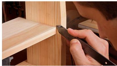
Mark the shelf notches. After milling the shelf to thickness and length, slip it into its dadoes as far as possible and make a knife mark at the shoulder. Then remove the shelf and cut the notches at the front edge.
