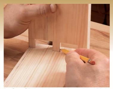
Transfer carefully. Hold the pins board against the tails board, lining it up carefully. Use a hard, sharp pencil to transfer the location of the pins, and then carry the layout around the end of the tails board.
