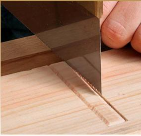
**Small shoulder guides the saw.** Rest a backsaw against the shoulder. Pull it backward to start the cut, and then tilt it to cut down to depth at the front edge before leveling the saw and finishing the stopped cut with short strokes.
