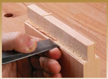
**Pare the shoulders.** Use a wide chisel to work your way across the shoulders, setting the tip of the chisel in the knife line each time.
