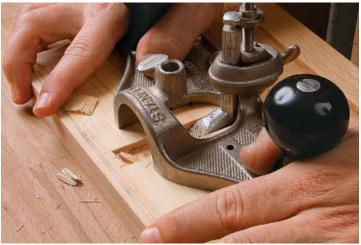
**Router plane finishes the job.** Lower the blade bit by bit to clean up the bottom of the dado. Use a chisel to chop the edges deeper if necessary.
