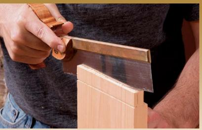
**Scribe and saw.** For both the shoulders and cheeks, use a knife to mark the layout and then keep the sawcuts on the waste side. To make the long cheek cuts, saw first into one corner as shown, come from the other side and saw into the other corner, and then finish the job with the saw level and the first two cuts guiding you.
