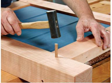
Drawbore the joints. Use straight-grained white oak for the pegs. The drawboring action eliminates the need for clamps. The pegs are trimmed flush later.
