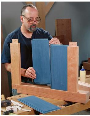
**Assemble the ends first.** Add the rails to one of the legs, then slide the panels in place. The second leg completes the assembly
