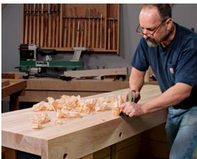
Attach the apron with the top in place. Resting the apron on the notches in the legs keeps it level, and makes it easier to get the first few clamps on. You'll need a lot of clamps. Plane it flush after the glue dries.
