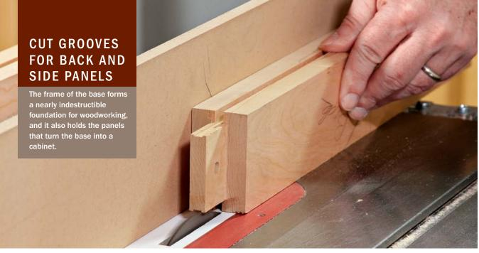
Throughgrooves are straightforward. Add an auxiliary face to the rip fence. Rip the groove in line with the tenon.
