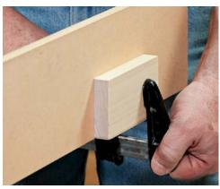
Stopped grooves need stop blocks. Clamp a block to the auxiliary fence (above). Place the trailing end of the leg against the stop, then carefully lower the leg onto the spinning dado set (right). Screwed to the outfeed table, a piece of MDF terminates the cut (below right). Turn off the saw before removing the leg.
