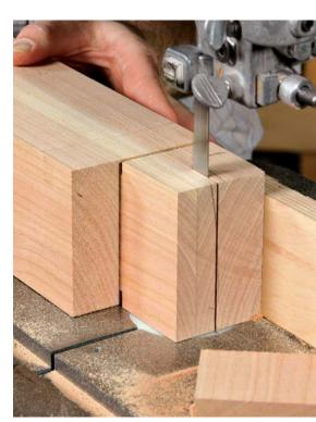
Two tools for stretcher tenons. Cut the shoulders at the tablesaw first. On the bandsaw, set the fence for the first cheek, cut it, then flip the stretcher to cut the second cheek.
