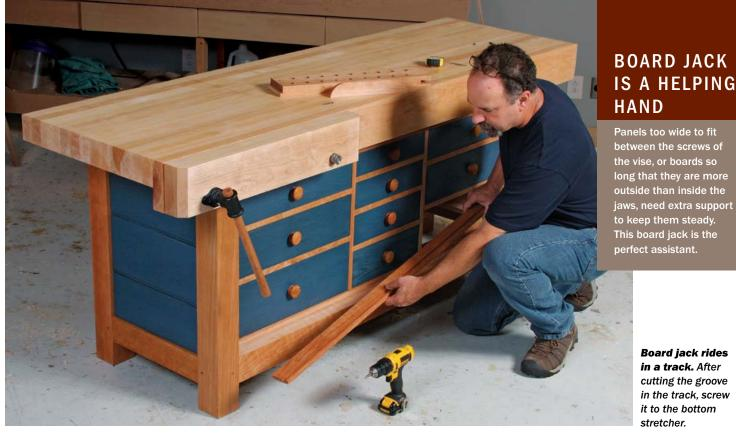
**Board jack rides** in a track. After cutting the groove in the track, screw it to the bottom stretcher.
