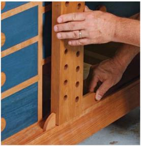
Big foot prevents racking. The long skate at the bottom of the jack allows it to slide more smoothly. Attach it with screws.
