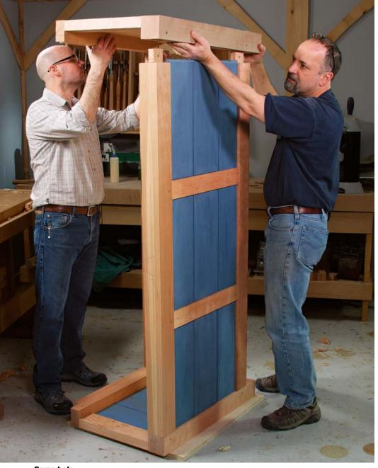
Some help required. After putting the front stretcher and assembled back into one of the ends, lower the second end into place. It's heavy, so ask a friend for help.
