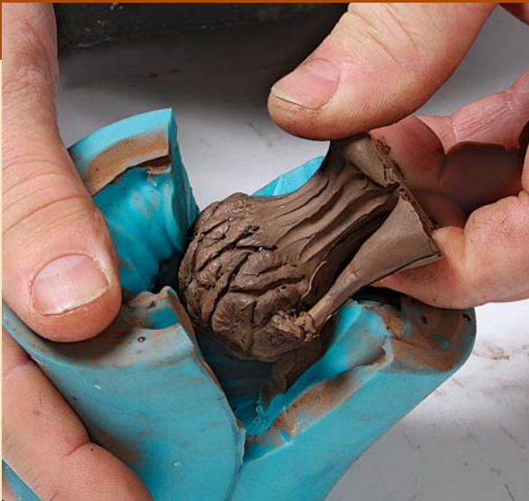
Easy out. The pliable silicone mold material makes it easy to remove castings.
