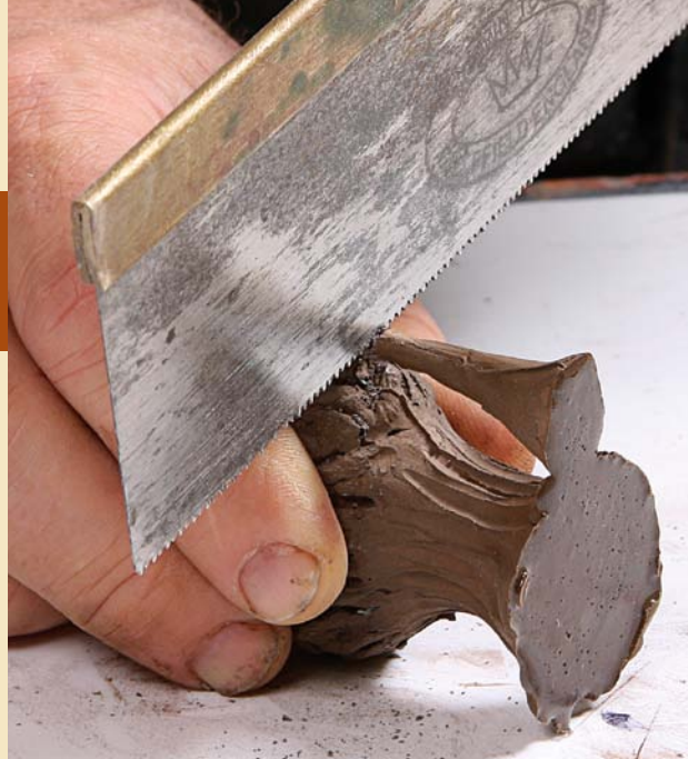
Trim the casting. The urethane resin can be worked like wood. Groove sawed off the vent, trimmed off the paper-thin flashing at the seams, sawed off some of the base, and then flattened it on a disk sander.
