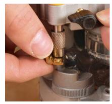
Set the depth. With the jig plate on a flat surface and the router resting on it, plunge the bearing-guided pattern bit through the notch until it bottoms out and lock it in. Then place a hinge leaf under the depth stop and tighten it in place.
