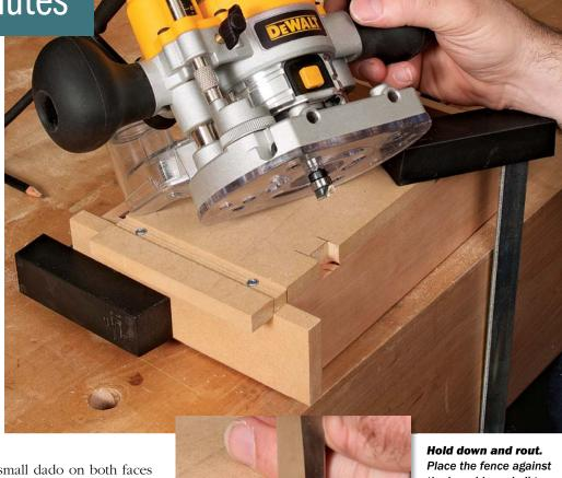
the box side and align the edge of the plate flush to the back of the box. Then clamp the jig in place. A quick pass with the router clears most of the waste. Keep the jig clamped in place. Square up the mortise with a chisel (left).
