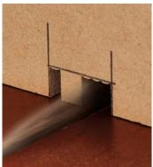
Then clear it out. Cut the hinge notch at the tablesaw with a miter gauge. Make the outside cuts first (leave the layout lines) and then remove the waste in between. For a flat bottom, slide the piece sideways over the blade while holding it against the miter-gauge fence.
