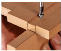
Quick-change fence. After routing one mortise on the box and one on the lid, simply remove the screws and flip the fence to the other side. The two remaining mortises can now be routed with the same settings as the first two.
