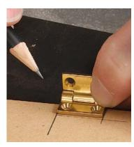
Lay out the hinge notch. After sizing the plate and cutting the dadoes for the fence, mark the notch directly from the hinge. Don't forget to account for the barrel.
