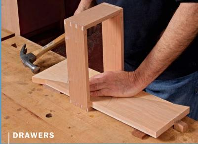
**Safely separate stubborn dovetails.** Two large opposing wedges force the sides apart while keeping them parallel, so there's no chance of cracking a pin.
