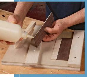
Ready to work. With the two fences in place, glue the edges of the workpieces and get them into position (above). A few light taps on the end of the wedge clamps this panel together (right). You can keep the pieces from springing up under the pressure by resting something heavy on top, like a handplane.
