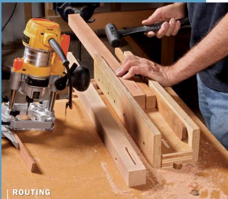
**Wedges won't get in the way.** Opposing wedges can clamp work for routing. Van Dyke uses a U-shaped jig to hold the workpiece for mortising and to support the router. A pair of wedges anchors the work solidly in the jig.
