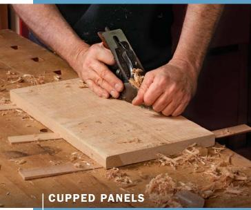
**Wedges for wobbly wood.** Use wedges to stabilize a cupped board or an oddly shaped workpiece on the workbench.
