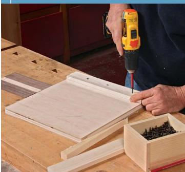
Build the jig. Screw one fence to a piece of 3/4-in.-thick plywood (above). To keep from gluing your workpieces to the jig, add packing tape to the top of the base. Then set the workpiece and wedge in place, and screw on the other fence (right).
