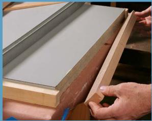
Even pressure on edging. A pine caul on each side helps line up the trim flush with the edges (above). Add a clamp across the end of the counter (right), spacing the bar about ¼ in. from the wood edging. Tap in wedges (below right) to apply pressure evenly along the glue joint.
