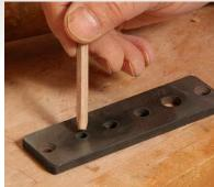
**Tapers result in better dowels.** Use a pencil sharpener to create a blunted point on both ends (left). This ensures that the blank will be centered in the hole when you begin (center). Also, as the blank exits the plate, the waste breaks off easily at the taper.
