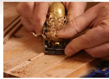
**Jig holds the blank.** A V-groove in the jig turns the blank 45°, standing the corner up for planing. Flatten the corner, but don't get too aggressive. If you plane too far, the dowel will have a flat side.
