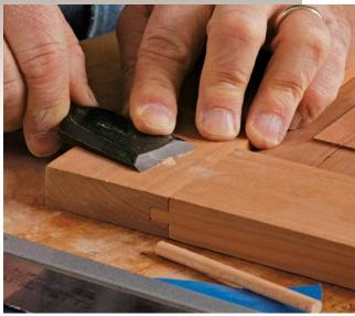
Trim flush. Pare the waste with a freshly sharpened chisel. Take it all in a single pass.
