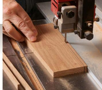
**Cut parallel to the grain.** A pencil line along the grain suffices as a guide (left). Clean up the newly cut edge with a handplane. To account for the blade's rough cut, rip the blanks just a hair over the final diameter (above).
