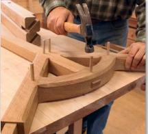
TOGETHER FOREVER A drawbored joint is pulled and locked together as the peg is driven home, making the joint ideal for hard-to-clamp assemblies like big table bases.
