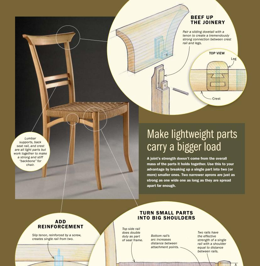
More than a decoration, cord wrapped around joint improves its strength, and because it's wrapped around the entire seat frame, it strengthens that, too.
