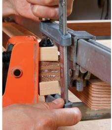
Elevate the work for glue-up. Godfrey supports the work on blocks and clamps each joint in both directions, ensuring that the joint fully seats (above). Finally, he clamps vertically across each joint (left) to ensure a good bond.
