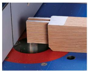
Fine-tune the fit. Godfrey uses a straight bit at the router table to trim the ends of the tenons (above). The table's fence is set to stop the cut at the bridle joint's shoulder. Then pare the miters so that their faces meet the shoulders of the bridle joint (right).
