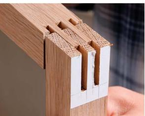
and the mating rail as you go. To position the fence, align the blade with the layout line of one of the tenon cheeks (see Step 1 above).
