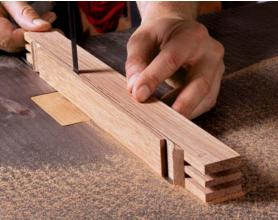
If the miters are tight but there are gaps in the bridle joints, you'll need to remove material from the miters, recutting them at the tablesaw or paring them slightly. If the bridle joints are tight and flush but the miters have gaps, use the router-table setup to take a little more material off the edges of the tenons.
