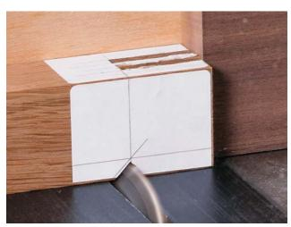
Angled cuts make the miter. Leave the blade a fraction low, to avoid cutting into the bridle joinery, but position the workpiece so that the miter's point will meet precisely with the bridle's shoulder (above). Trim the excess at the bandsaw (right), guiding the cut with the fence.
