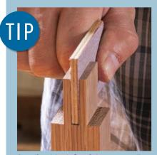
Sanding block for tight spaces. To ease a too-snug fit, Godfrey carefully sands using P120-grit paper glued to a thin plywood sanding block.
