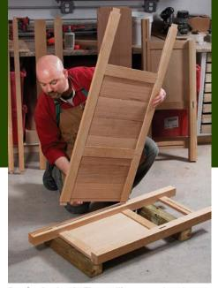
**Put in the back.** The mullions are already glued in place. Because the slats float in the grooves, hold them in the side panel as you lower the tenons into their mortises.
