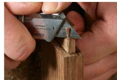
**Quick tenons with a dado set.** Cut the end of the tenon first. Register the opposite end of the board against a stop block to cut the shoulder (left). This ensures that all of the tenons are the same length. Paolini uses a utility knife to knock off the corners (above), allowing the tenons to fit into the rounded mortises.
