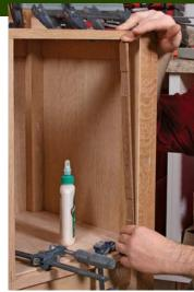
**Set the subtop in place.** The filler strips are glued to the end assembly (left). After screwing the subtop to the drawer divider assembly, lay (do not glue) the false bottoms on the case bottom (center). Then glue hinge strips—mortise them first—to the legs (right). Finally, place the top on the case (below), and secure it from below with screws.
