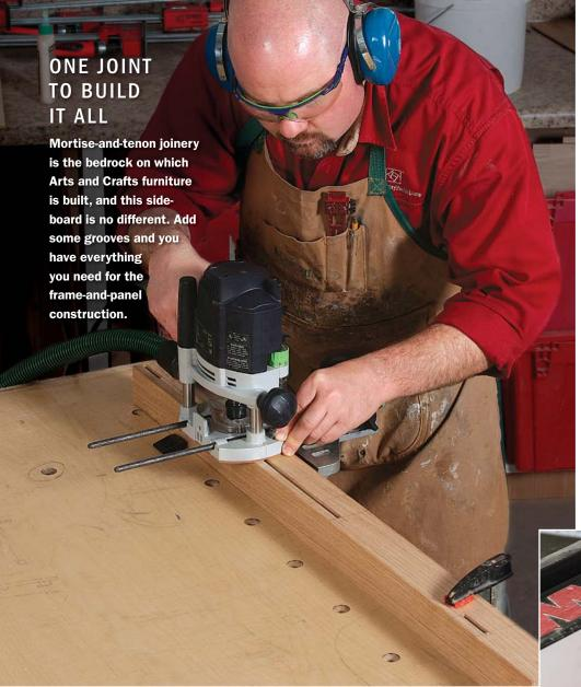
**Rout the mortises and stopped grooves.** Use a <sup>1</sup>/<sub>4</sub>-in.-dia. spiral upcut bit. The router's edge guide locates the bit and keeps it cutting straight (above). Cut through-grooves for the panels at the tablesaw (right) using a standard-kerf blade. Make the groove in two passes, registering the opposite face on the fence for the second cut. This centers the groove on the part's thickness.
