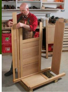
The shelf and plate rack come next. Then put in the remaining back slats, and spread glue on all of the exposed tenons before adding the second end assembly.
