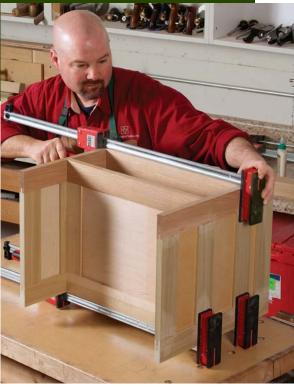
**Build the drawer divider assembly.** After gluing up the horizontal dust frames and panels, glue them into the dadoes cut into the frame of the vertical partitions (above).
