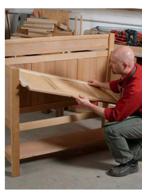
**Drop in the case bottom.** Attach it by screwing up through the front rail. In the back and on the sides, it simply rests on the lower rail of the frame.
