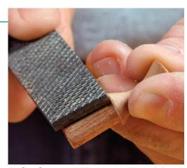
**Perfect for tenons.** When a turned tenon is just a bit too big, a file with a safe edge is the best tool for trimming without damaging the shoulder.
