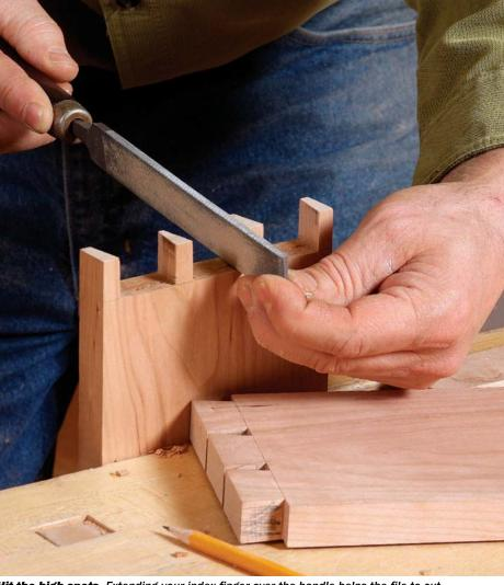
**Hit the high spots.** Extending your index finger over the handle helps the file to cut in a straight line so that you don't round over the pin. Pinch the other end of the file between your fingers.
