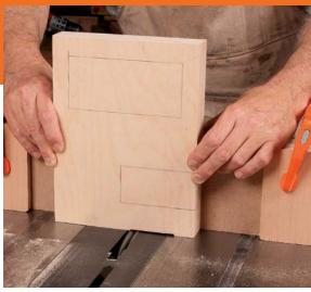
Relieve the bottom of the stretcher. Latta uses a dado blade. He attaches a tall fence between two miter gauges and clamps on blocks to stop the cut 1 in. from each side.
