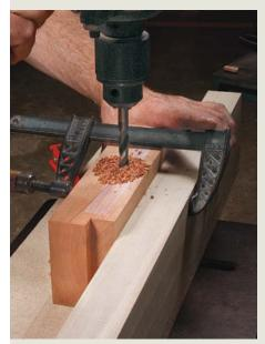
Drill for the dowel. Clamp a backer block to the pivot block and drill a 3/8-in. hole on the seam to create a half-round channel for the dowel. Then drill the wooden jaw pads the same way.
