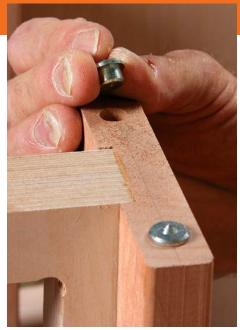
**Pop in a pair of dowel centers.** Latta uses dowels to register the front of the benchtop flush with the legs. To locate the dowel holes in the top, he uses dowel centers.
