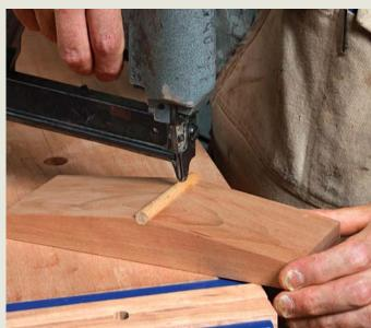
Attach the dowel. Fasten the 3/8-in. dowel to the block with glue and a few small brads.
