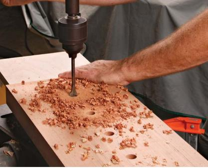
**Drill the dog holes.** To avoid blowout, Latta uses a spade bit in the drill press. He sets the depth stop for just after the point comes through, then flips the benchtop and finishes from the other side.
