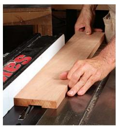
**Groove the leg post for the stretcher.** Latta cuts the groove a little at a time, testing the fit with a stretcher as he goes.
