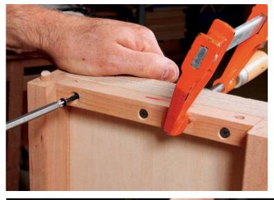
Cleats keep it all together. Mount the cleats ½2 in. shy of the top (left), to ensure the legs are pulled tightly against the top. Put the legs in place, and screw them down. Sink the screws that connect each cleat to the top (below).
