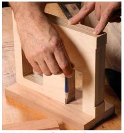
Mark the leg post for the mortise. Use the stretcher to transfer the location of the clamp mortises onto the posts. Cut the mortises using a scrollsaw.
