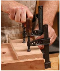
**Get the vise at the right height.** Glue on a spacer block to locate the top of the vise ½s in. below the benchtop.
