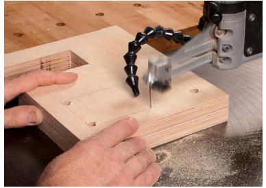
Cut out the mortises and notches. Drill the four corners of the mortise for the vise hardware and cut the sides on the scrollsaw. Make the long cuts for the notches on the bandsaw, then connect the ends on the scrollsaw.
