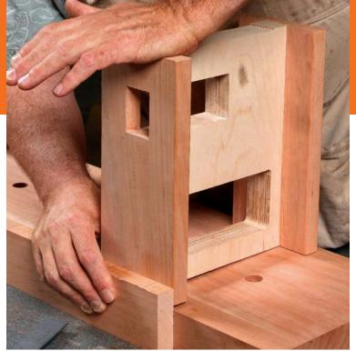
pressure on these points. A flat scrap of wood helps get the legs flush with the front of the benchtop. Then just add pressure. The pointed dowel centers will create a perfect set of
