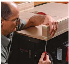
Make an adjustment. Figure out which way the fence is skewed, and then loosen the screw in the slotted hole, give the fence a tap in the right direction, and retighten. Make as many test cuts and adjustments as you need.
