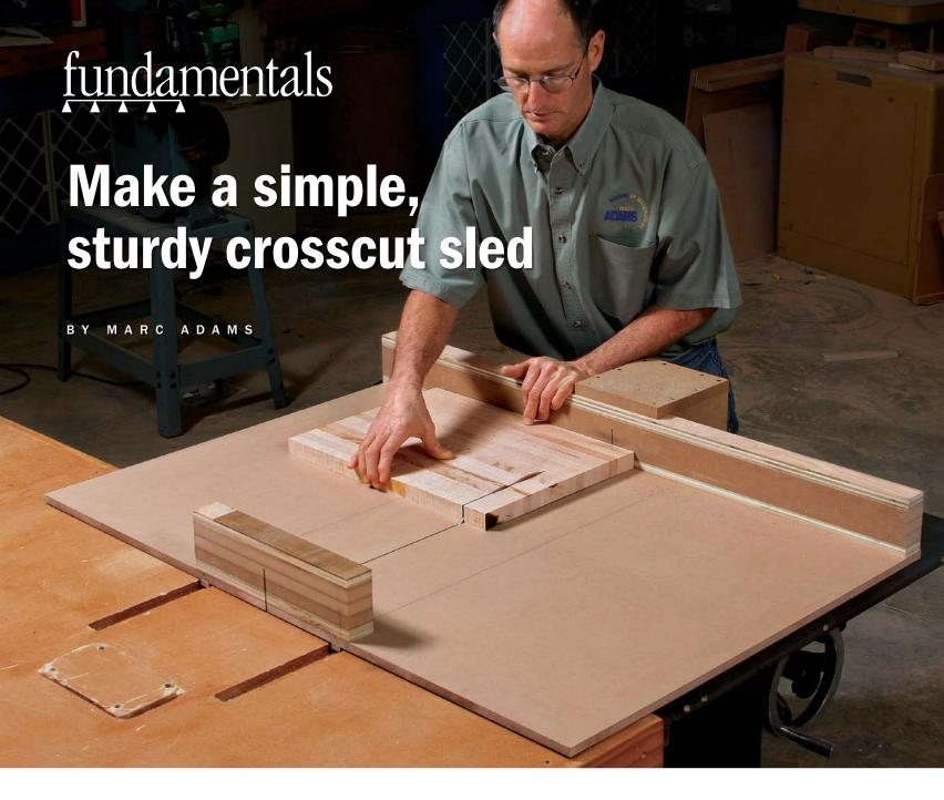
hile your tablesaw's miter gauge will work OK for cutting smaller workpieces to length, nothing controls large and small work better than a good crosscut sled. With it, you'll get furniture-quality crosscuts as well as clean, accurate dadoes, rabbets, bevels, and much more. To explore the possibilities of this essential jig, check out my article, "Cut Precise Joints on the Tablesaw," in FWW #235.
