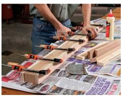
Give up and clean up. Rip the strips of plywood and MDF 13/4 in. wide, and then glue and clamp them (above) to make tall blocks for the short and long fences. After the glue dries, scrape off the squeeze-out, and then clean up the edges on the jointer (right) and planer.
