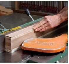
Front fence needs extra care. On the long front fence, lightly joint one of the plywood layers square with one edge of the sandwich, and keep track of those two good surfaces.
