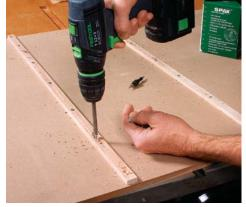
Flip and fasten. Now flip over the sled and drill, countersink, and drive screws (above). The nails will hold the runners in alignment while you lock them down permanently. Next, add the back fence (right). Align it with the edge of the sled, and screw it into place. Just keep the screws away from where the blade will pass through.
