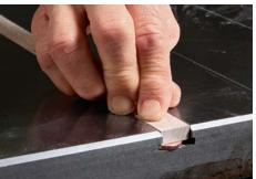
Shim them up. The runners are thinner than the slots are deep, and you'll need to shim them flush with the surface for the next step. Adams used pennies as shims (above). After aligning the front of the sled and the runners with the front edge of the saw table, mark lines on the base over the centerlines of the runners, and drive a few short brads into each of them (right).
