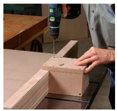
**Don't forget safety.** Attach a box to the front fence to cover the spot where the blade emerges, and be careful not to push the sled too far forward in use.
