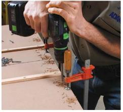
**Lockdown.** When there are no gaps in your test pieces, flip the sled over and drive a row of screws into the fence to lock it in position.
