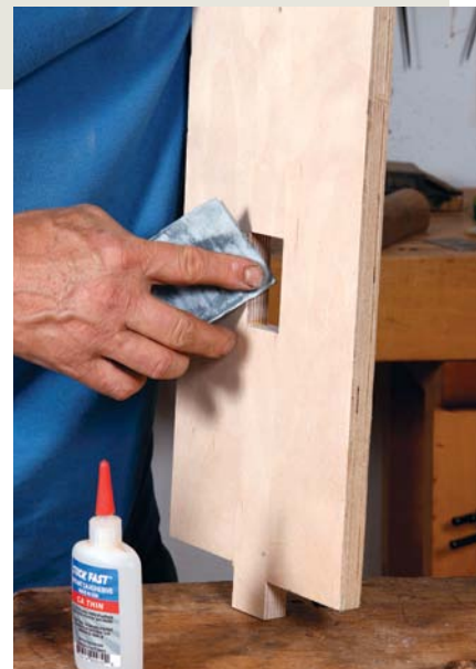
An accurate, durable guide slot. Boggs makes the template by ripping a piece of plywood and reassembling it. He coats the edges of the guide slot with cyanoacrylate glue and sands them.
