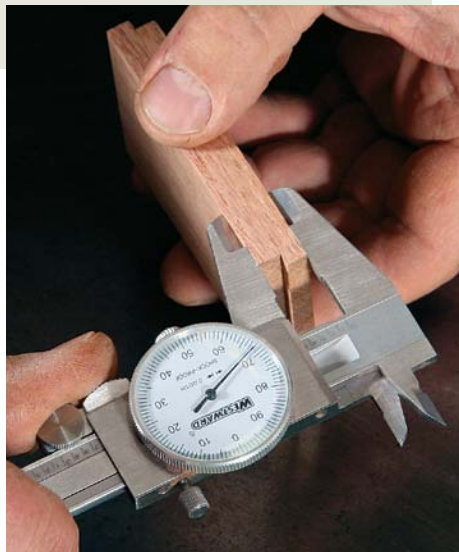
Measure a kerf. To find the width of the bandsaw kerf, use a micrometer to measure a scrap before and after it's been sawn down the middle.
