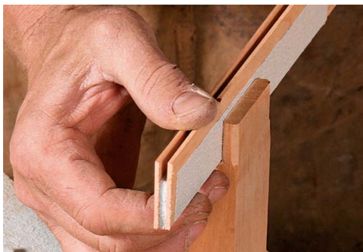
Tiny taper. A few fine shavings with a block plane create a subtle taper on the ever-so-slightly oversize rail. The taper makes insertion easier and ensures a seamless glue line.
