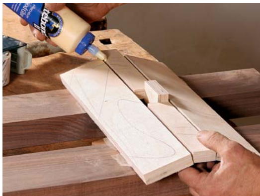
An accurate, durable guide slot. Boggs makes the template by ripping a piece of plywood and reassembling it. He coats the edges of the guide slot with cyanoacrylate glue and sands them.
