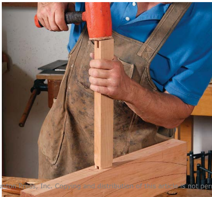
Fit, then shape. After dry-fitting the joint, Boggs will disassemble it and shape the parts before final glue-up.
