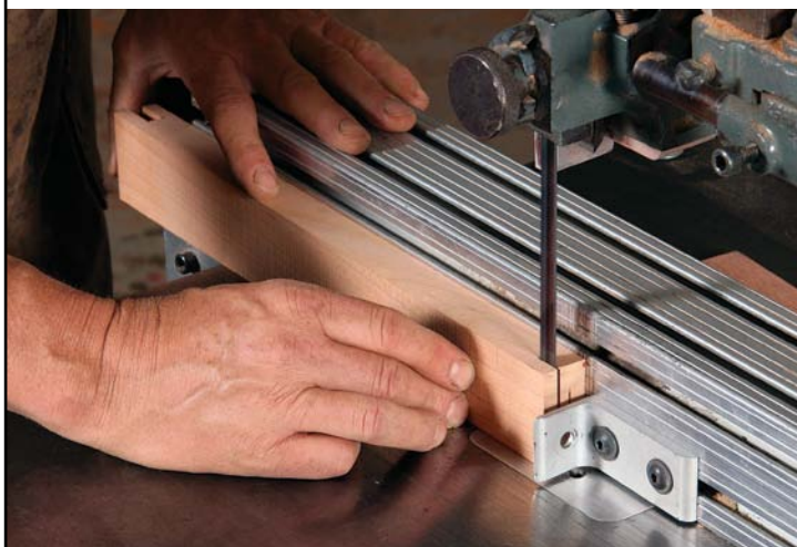
First cheek. Cut the cheek of the far tenon with the workpiece riding against the bandsaw fence. A stop controls the depth of cut.
