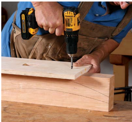
Clamped with a fence. When there are multiple mortises to cut, or when it's not practical to screw the template to the workpiece, you can attach a fence to the template and clamp it to the workpiece.
