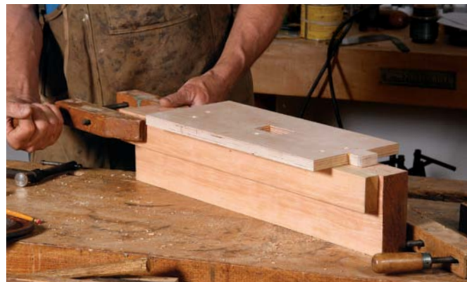
Clamped with a fence. When there are multiple mortises to cut, or when it's not practical to screw the template to the workpiece, you can attach a fence to the template and clamp it to the workpiece.
