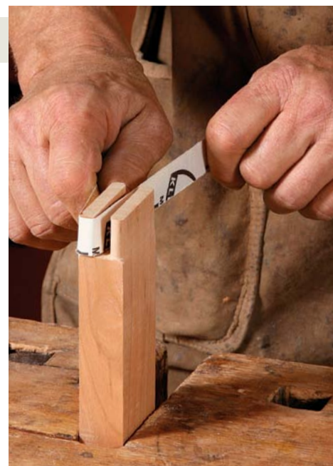
Round the tenons. Sandpaper used with a shoeshine stroke makes quick work of knocking the corners off the tenons so they fit the rounded corners of the routed mortises.
