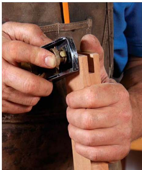
Tiny taper. A few fine shavings with a block plane create a subtle taper on the ever-so-slightly oversize rail. The taper makes insertion easier and ensures a seamless glue line.
