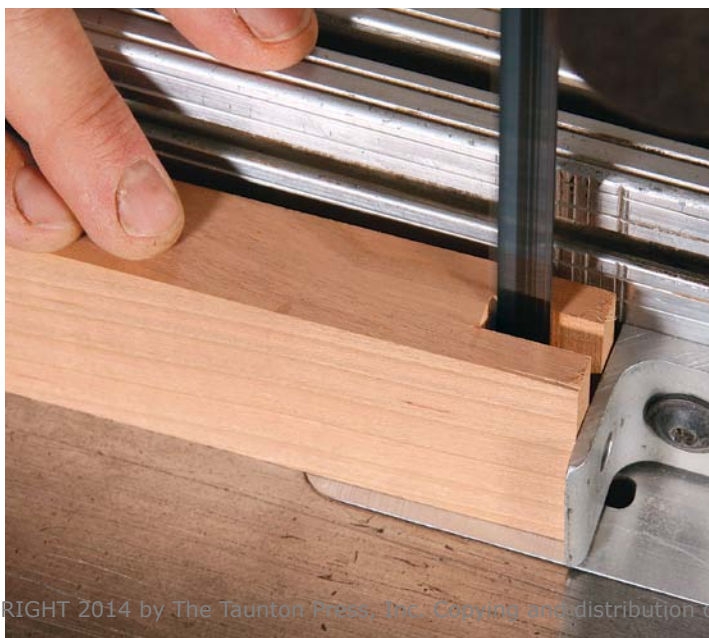
First cheek. Cut the cheek of the far tenon with the workpiece riding against the bandsaw fence. A stop controls the depth of cut.
