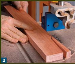
**Cut.** Bandsaw right up to the pencil line, leaving just a little waste for the router to remove.
