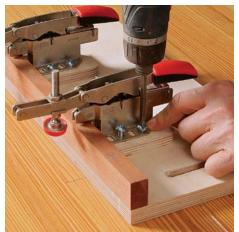
Bolt on the clamps. The upward force of the clamps could be too great for screws.
