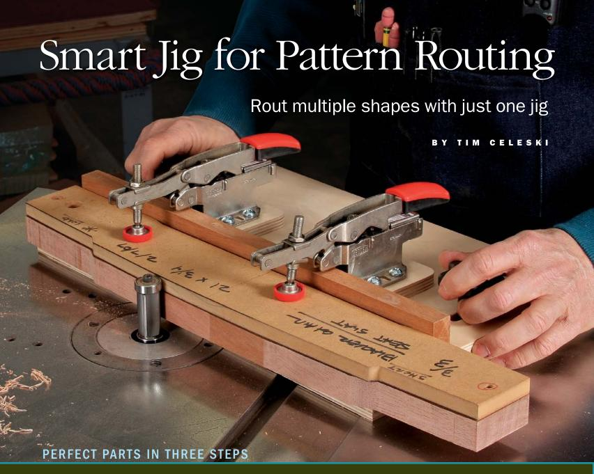
If you need two or more of a workpiece that has a curve, bend, or decorative shape like a cloud lift, the smartest way to make them is with a pattern and router.
