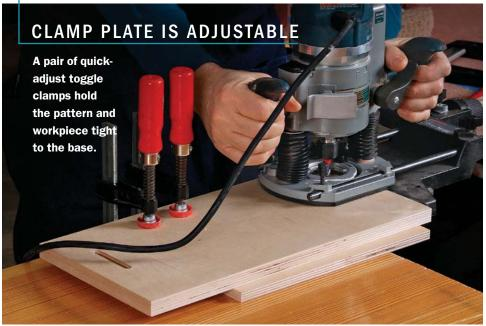
**Slots allow for movement.** Make them  $\frac{1}{16}$  in. wider than the diameter of the knob's threaded shank so that you can angle the clamp plate differently to use the jig for a wider range of patterns.
