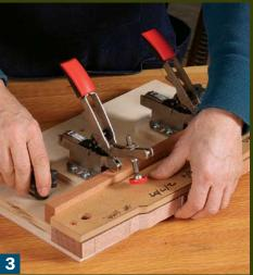
**Rout.** With the pattern and workpiece overhanging  $\frac{1}{2}$  in., lock the clamp plate to the base, then clamp in the pattern and workpiece.
