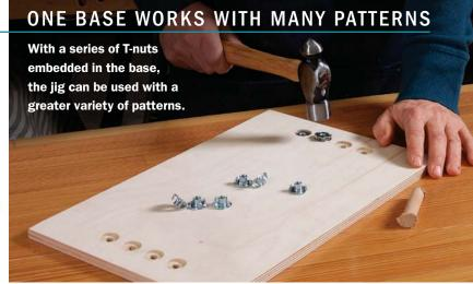
**Knock in the T-nuts.** Counterbore the underside to allow the T-nut's flange to sit just below the surface. Then drill all the way through for the T-nut's shaft. Celeski uses a dowel (foreground) to knock the T-nuts below the surface of the base.
