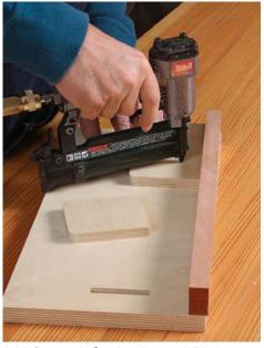
**Add riser pads for the clamps.** With the fence resting in place, glue and nail the pads to the clamp plate.
