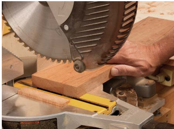
Bevel the ends. A miter saw cuts clean bevels on the ends of the front stretcher.
